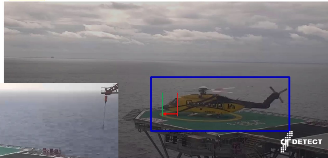
Aircraft incorrectly positioned on the TD/PM within TLOF
