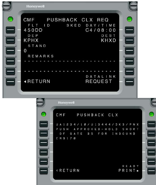
Pushback Clearance Request and Response
